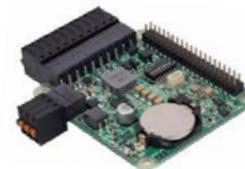
The RAS function expansion card adds RAS functionality, RTC functionality, and 8–28 VDC power supply input functionality to the Raspberry Pi. This HAT-sized expansion card connects via a 40-pin header for stackable connection and provides the Raspberry Pi with the enhanced scalability and maintainability required for industrial computer applications.
